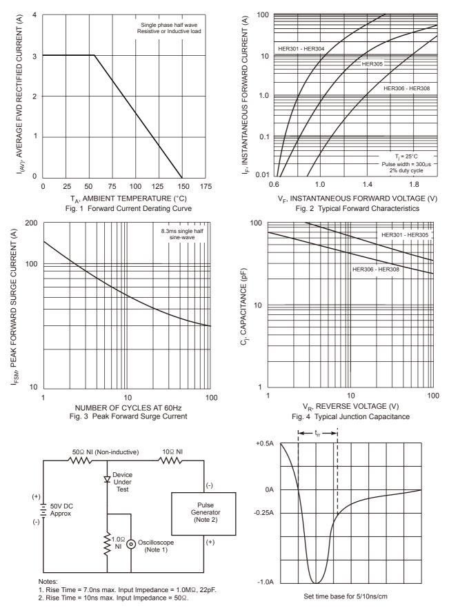
Fig. 5 Reverse Recovery Time Characteristic and Test Circuit
